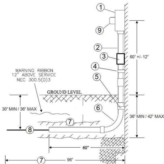
Excavation for foundation must be backfilled and tamped by customer prior to conduit installation to prevent further settling.
